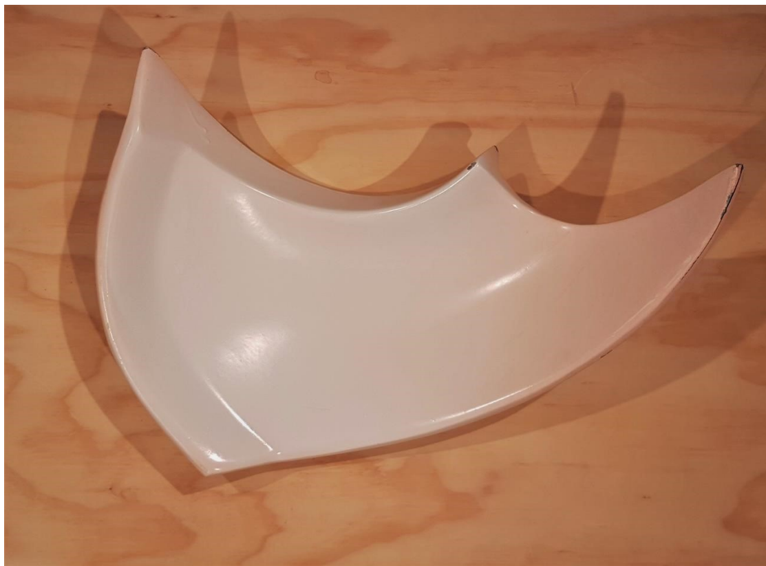
Blade of the 5 kW model, top view.
